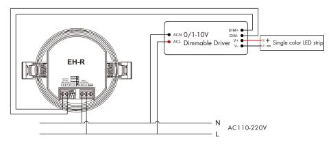
• Used as dimmer or switch, connect with 0/1-10V dimming driver (use AC OUT)
