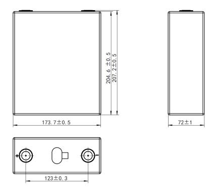
Figure 4. Lithium-ion cell three views (unit: mm)
