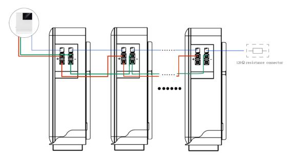
Figure 9. Connect the internal cables
