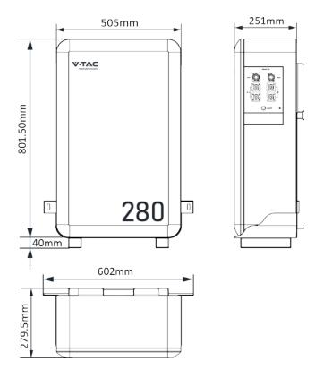
Figure 2. V-Power S14 dimensions (unit: mm)
