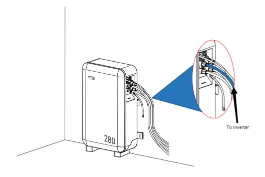
Figure 10. Connect the external cables
