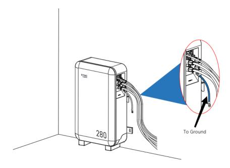
Figure 7. V-Power S14 grounding
